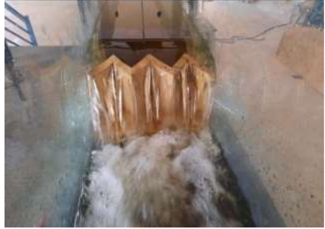
Equilateral Triangle Labyrinth weir
