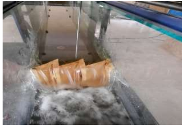
Right Triangle Labyrinth weir
